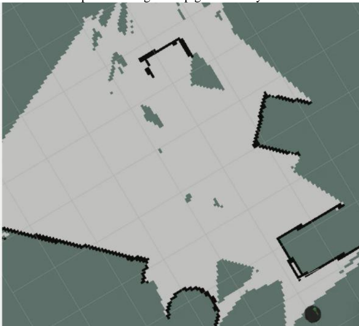
Figure 2: a 2D grid map. The black spaces represent obstacles, the grey represents safe space for navigation.
